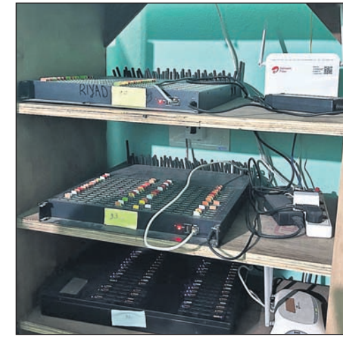
SIM BOXES ARE USED TO HIDE ORIGINAL PHONE NUMBERS AND ARE OFTEN EMPLOYED FOR CYBERCRIME, HATE SPEECH, TERRORIST ACTS, EXTORTION, AND OTHER ILLEGAL ACTIVITIES, POSING CHALLENGES FOR LAW ENFORCEMENT AGENCIES
