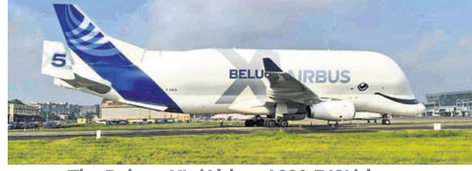
The Beluga XL (Airbus A330-743L) is one of the large transport aircraft designed by Airbus to carry oversized cargo, primarily aircraft components such as wings and fuselages
